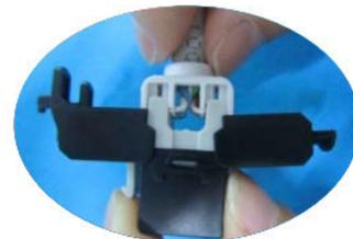
The tiny teeth on the outer side of IDC slots.
