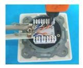
Adjust the gap on the cover to fit the cables. Latch the snag (the marked part in the following picture) to the hole on the body and then fasten the screw.
